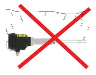
In case vapour splash cable potting points, insulation problem may cause.
