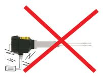
Excess current , to be drawn as a result of direct connection to motor, may burn relay of switch
