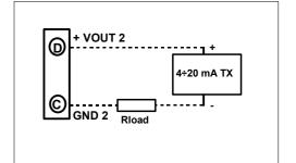
Note: terminals A and B not connected (NC).
