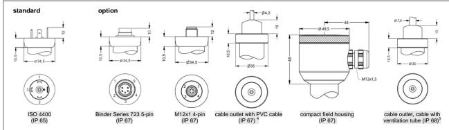
standard: 2 m PVC cable (without ventilation tube, permissible temperature: -5 ... 70 °C)
