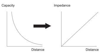
Excitation applied between 10KHz...250KHz based on length for all our models.  $\varphi$  =2xpxf) Linearity error that may be caused by conductivity component (R) effect is prevented by electronic circuit design and mechanical design. Reduced to a level lower than 1ppm, acceptable as zero.
