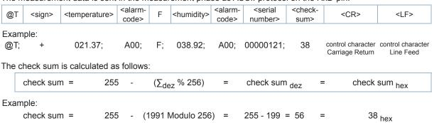
The check sum is not transmitted as a hexadecimal character with 1 byte, but is translated into readable digits with 2 bytes. Through the comparison of the transmitted check sum with a check sum calculated at the read-out point, the user has the opportunity to check whether the transmission of the data is error-free.
