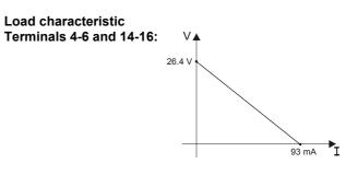
NOTE: The electrical parameters on terminals 6-5 and 16-15 are within the limits defined in the par. 5.7 of the standard EN 60079-11 relative to "Simple Apparatus".
